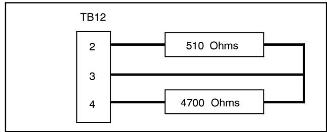
**Figure 9-16** Throttle Emulator (or Equivalent)
