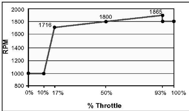
**Figure 9-12** Isochronous Governor (55-99EOZD and 40-80EFOZD Models)
