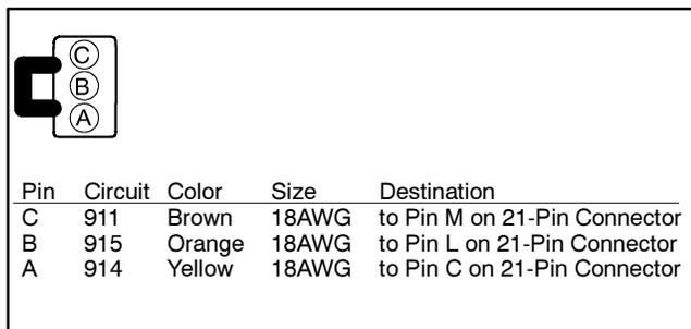
**Figure 9-15** Analog Throttle Potentiometer
