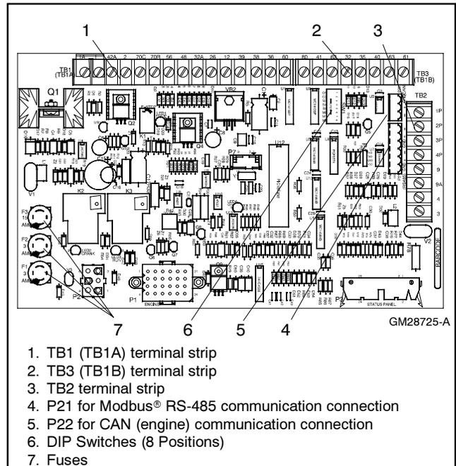
**Figure 8-7** Controller Circuit Board with DIP Switches
