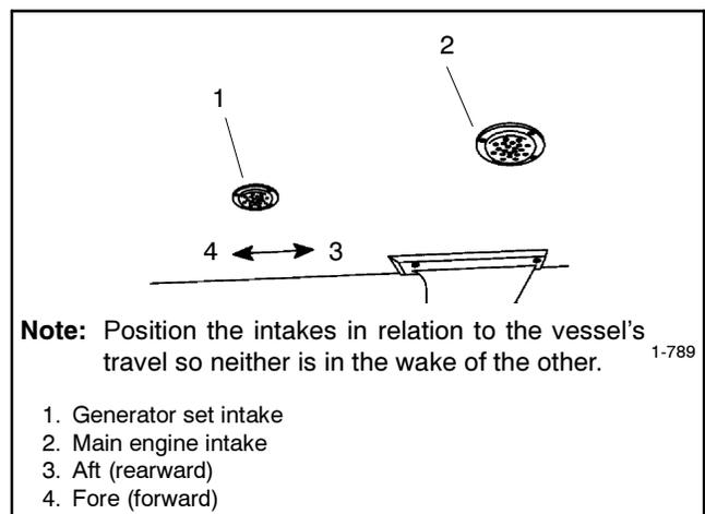
**Figure 3-3** Intake Strainer
