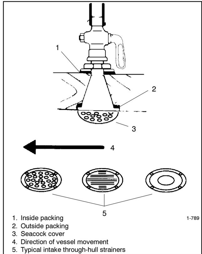
**Figure 3-2** Seacock Installation
