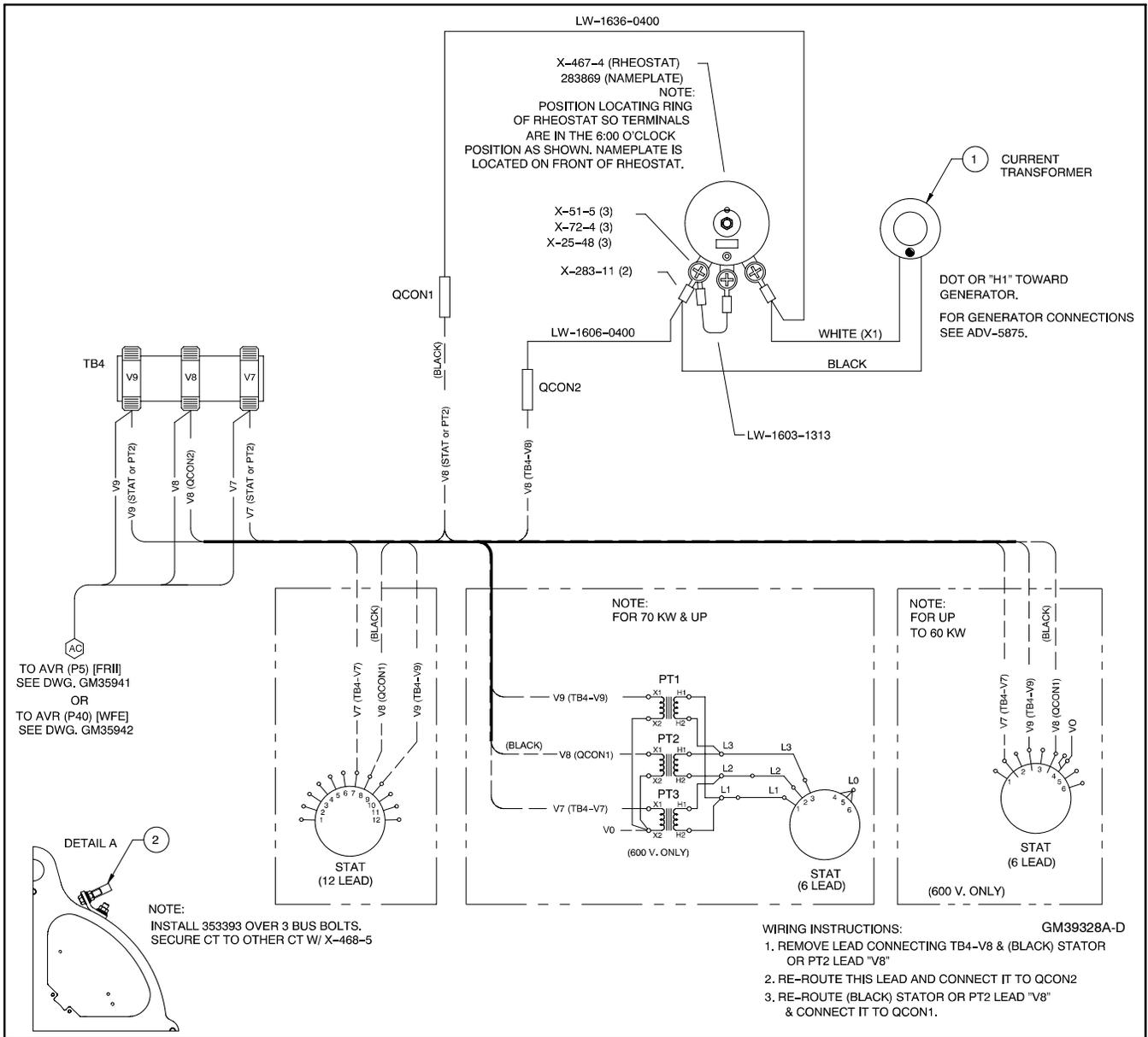
**Figure 9-20** Reactive Droop Wiring Diagram
