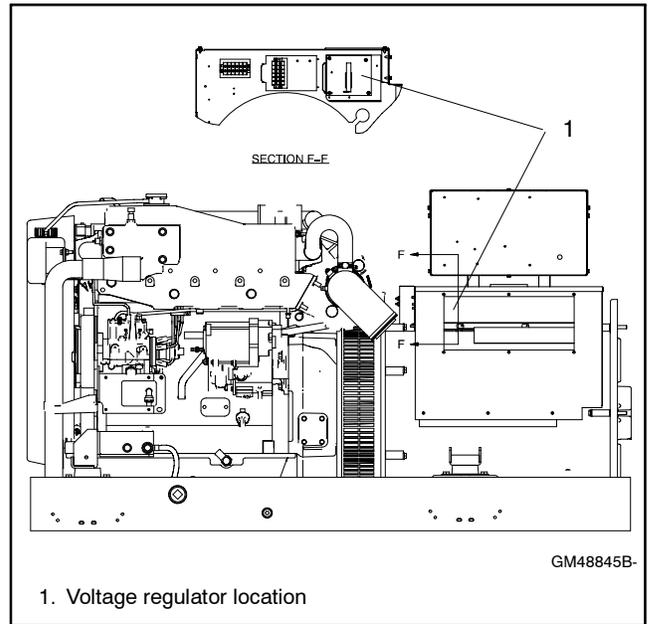
**Figure 9-23** Kohler FR™ II Enhanced Voltage Regulator Location
