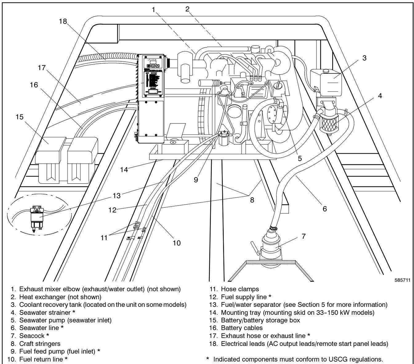
**Figure 1-1** Typical Generator Set Location and Mounting (Without Sound Shield)
