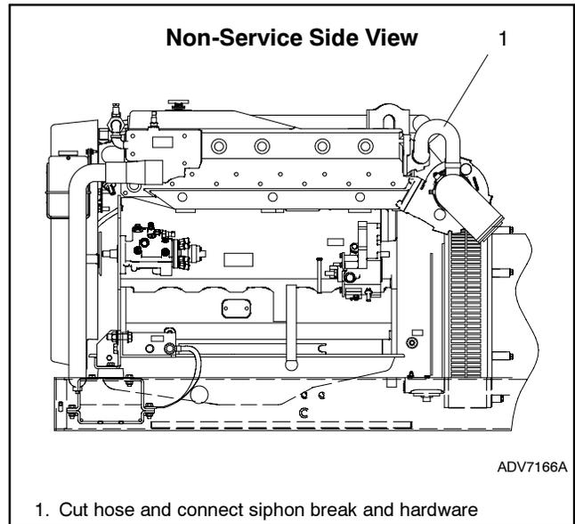
**Figure 4-4** Siphon Break Connection (Typical for Non-Sound Shielded Units)
