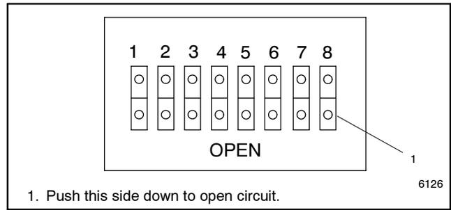
**Figure 8-9** DIP Switch Open Position
