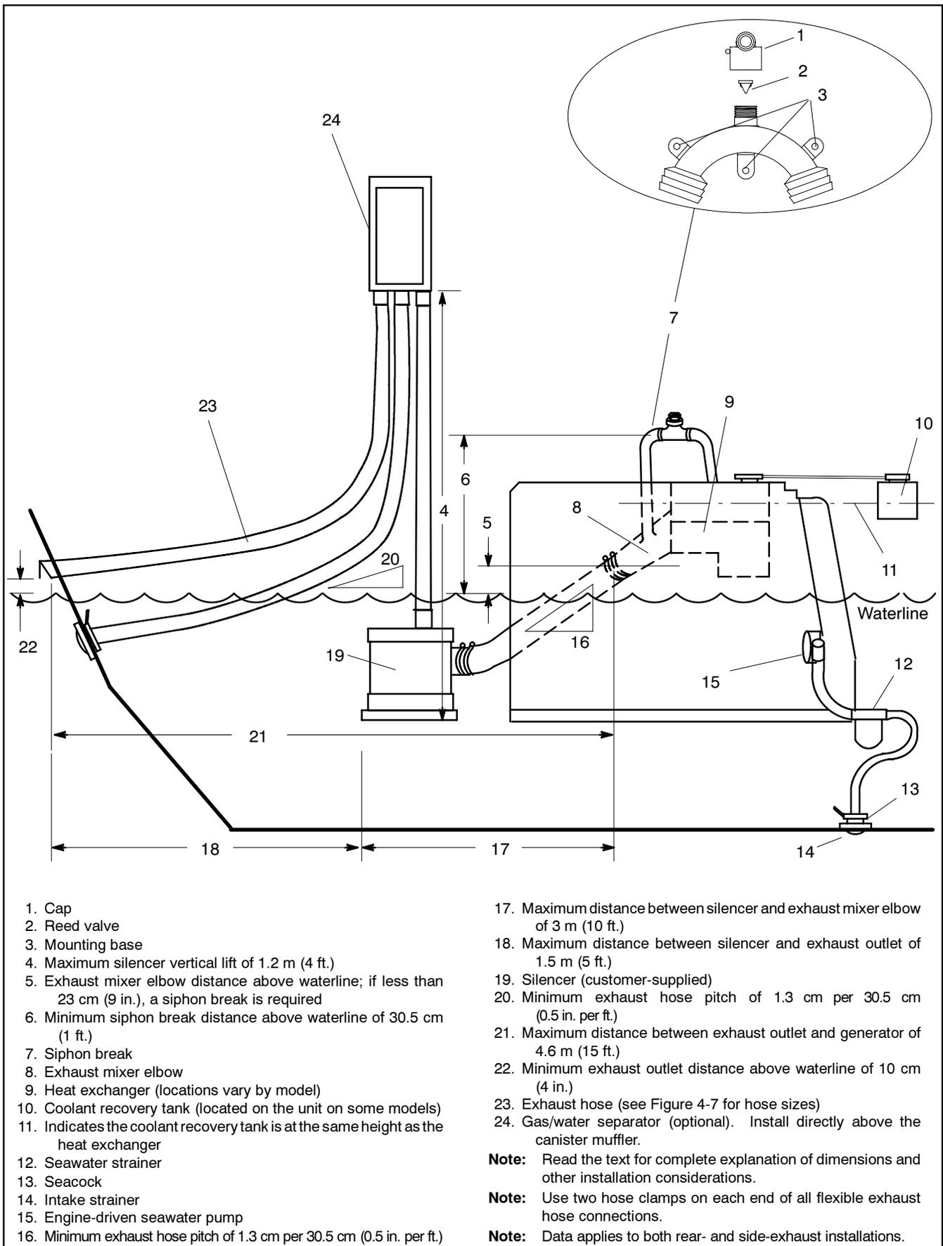
**Figure 4-5** Typical Mid- and Below-Waterline Installation with Optional Gas/Water Separator
