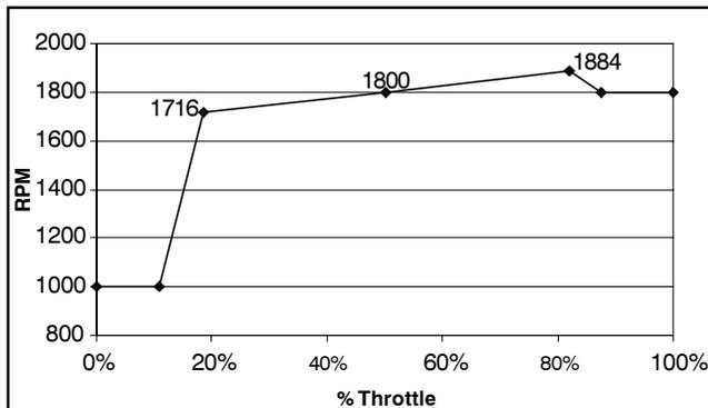
**Figure 9-13** Isochronous Governor (125-180EOZD and 100-150EFOZD Models)
