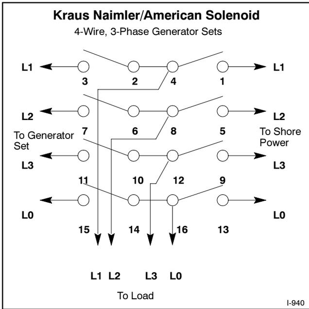
**Figure 8-2** Marine Manual (Ship-to-Shore) Transfer Switch, continued
