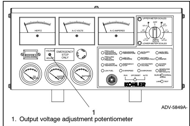
**Figure 8-5** Voltage Adjustment
