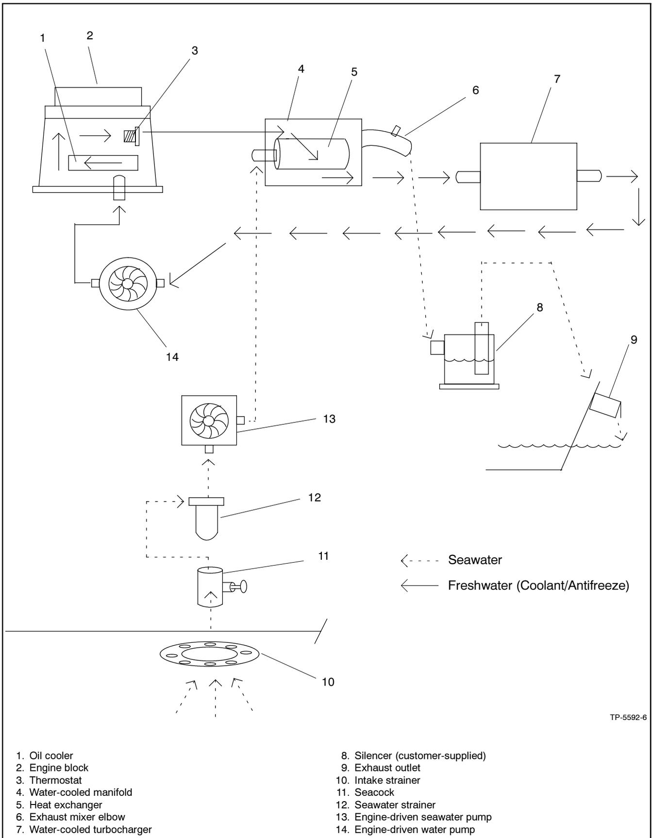
**Figure 3-6** Typical Closed/Heat Exchanger Cooling System (40-180EOZD/33-150EFOZD Models)
