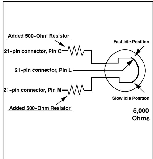
**Figure 9-18** Potentiometer Without Mechanical Adjustment Stops
