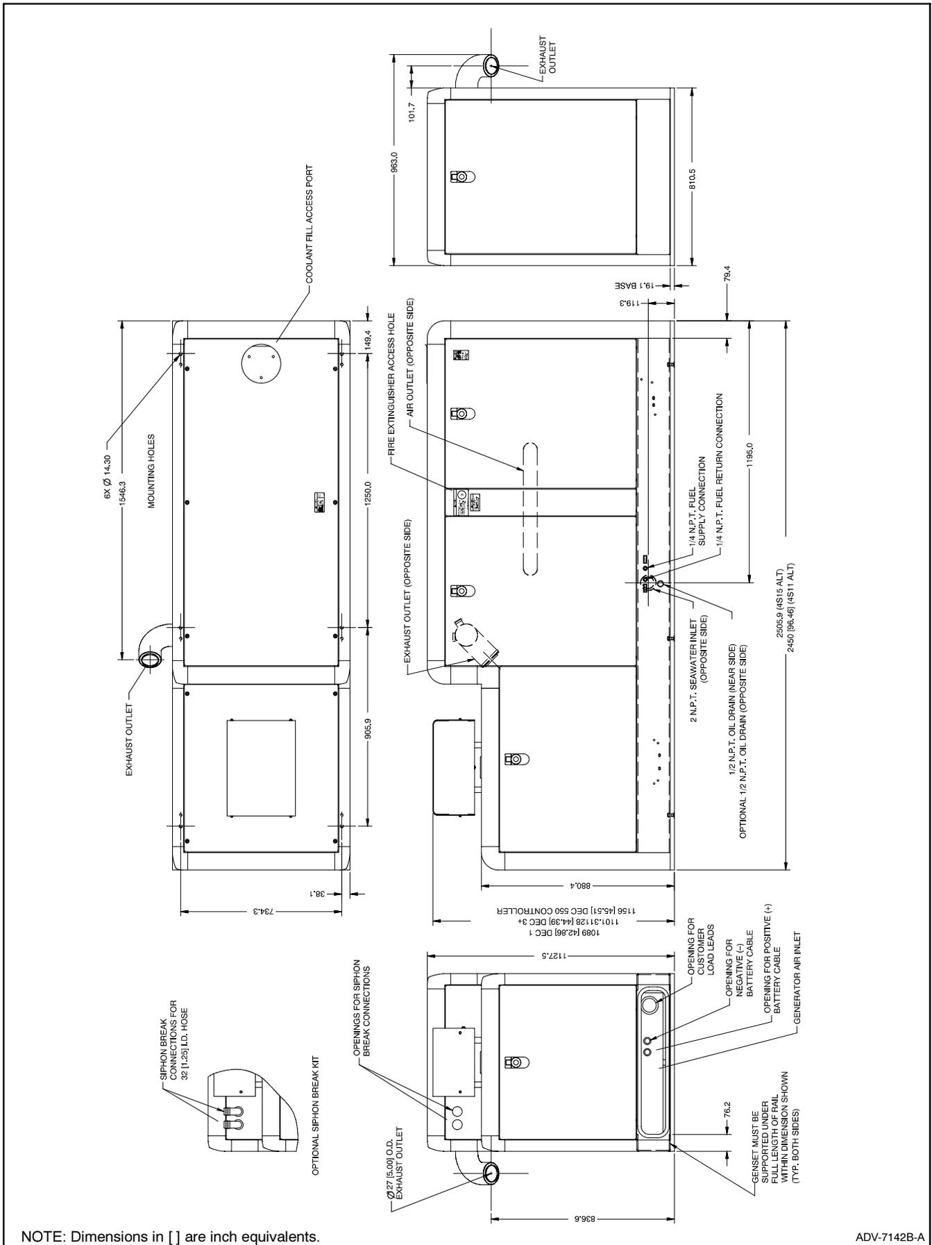
**Figure 7-18** Dimension Drawing, 125/150EOZD and 100/125EFOZD with Sound Shield
