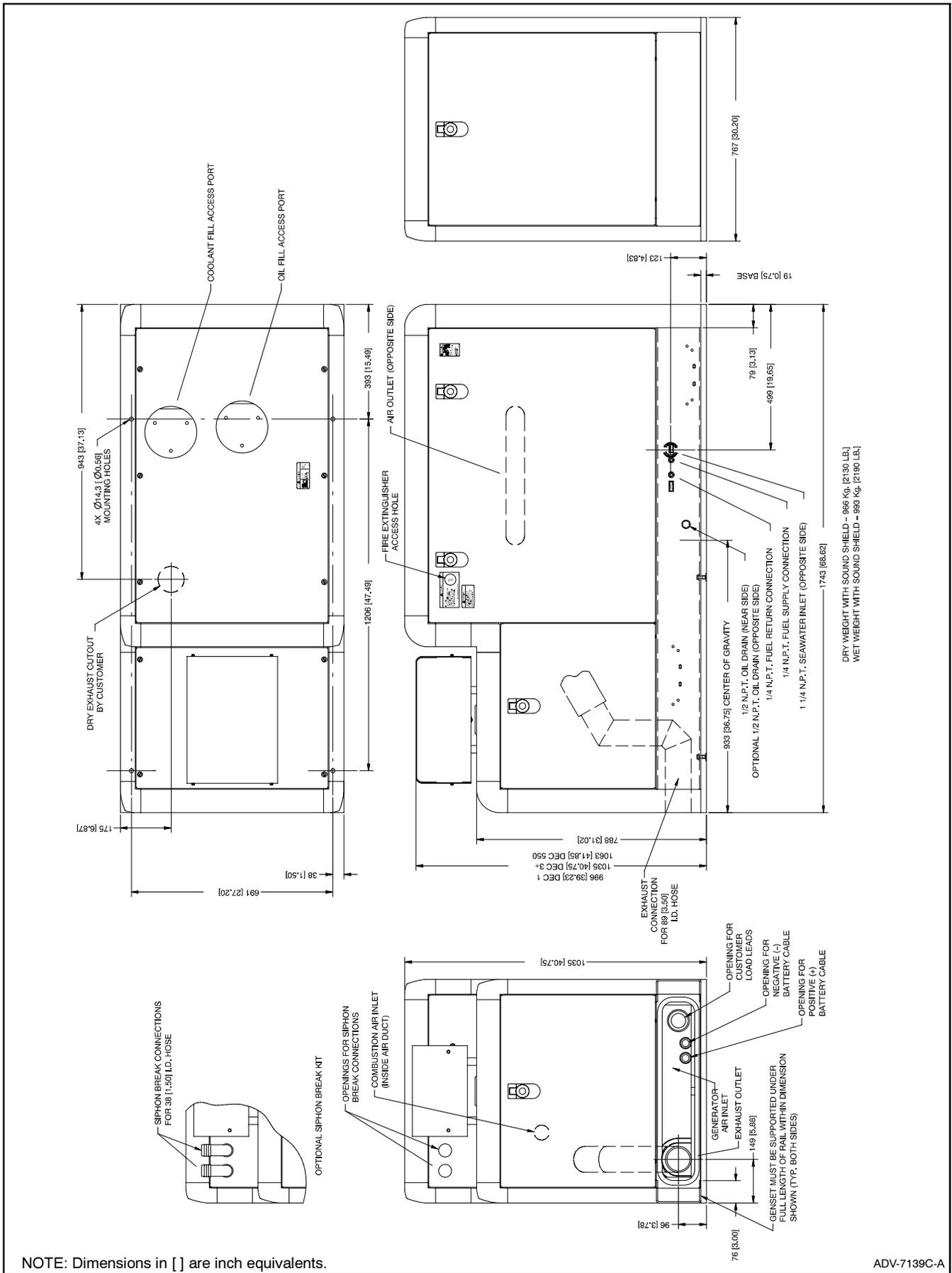
**Figure 7-4** Dimension Drawing, 40EOZD and 33EFOZD with Sound Shield
