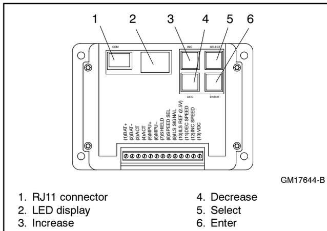
Figure 9-3 Governor Controller Functions
