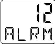
If the fuel remaining value drops below the fuel alarm value, the alarm will sound and the "ALRM" will flash.
