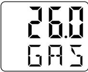
Press and hold both up and down buttons together for two (2) seconds.
