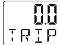
The Trip log value may be reset without changing the Total log value. If the Total log is reset to zero (0), then the Trip log will automatically reset to zero (0).
